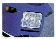
Halogen Headlight and Maintenance-free battery The RG500l' sports a 60/55W rectangular halogen headlight. The winkers are integrated into the fairing. The RG500F also features a fully sealed battery that requires no troublesome topping up with battery fluid.
