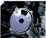
Heart-Grabbing Pickup from Low to High Engine Speeds with the SUZUKI INTAKE POWER CHAMBER. What the SUZUKI INTAKE POWER CHAMBER does is to increase intake efficiency and to improve power output and fuel consumption at low
